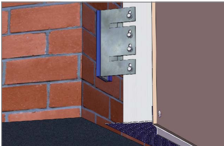
Bottom Drip & Vent onto FastFrame Aluminium trim :AL/BD/86 uPVC trim :088P Vent :AL/VENT/30/100 Fixing :RIVETS/18 Gasket :090/35N
