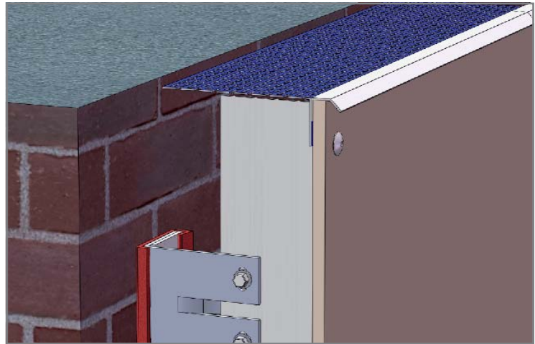
Top Drip & Vent onto FastFrame Aluminium trim :AL/AD/6/11 uPVC trim :RD91 Vent :AL/VENT/30/100 Fixing :RIVETS/18 Gasket :090/35N
